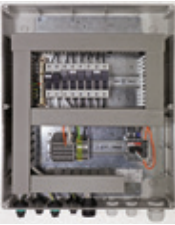
W3E - THREE-PHASE ELECTRICAL PANEL FOR 400V-3-50HZ EC FANS Electrical panel for EC fans with plastic casing, fuse protection for groups of fans and external control 0-10V.
